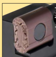
Modified cartridge with approach angle of 93^\circ (difference of 6^\circ )
