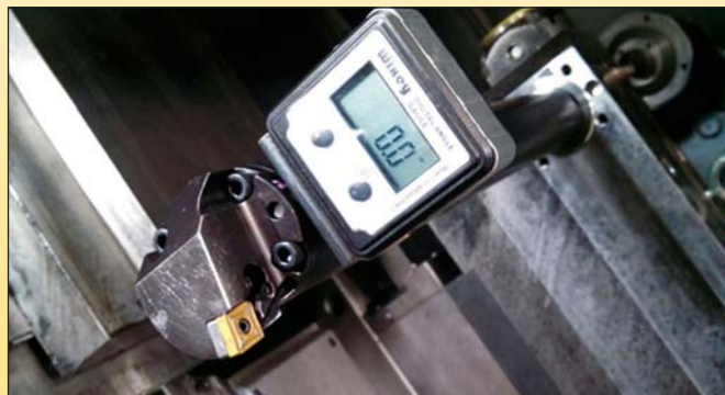
Figure 4: Aligning the boring bar
